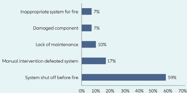
It is clear from the graph above that inadequate inspection and maintenance of sprinkler systems are directly related to 76% of the sprinkler system failures.
