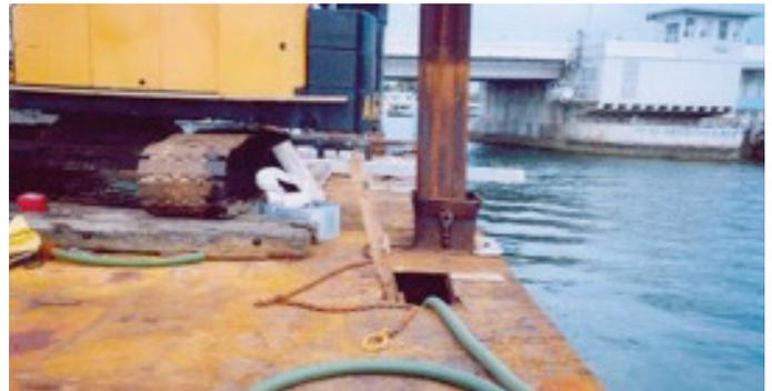
Note hole cut in deck and the portable pump & hose on deck. Barge must be regularly pumped to keep the compartment from flooding.
