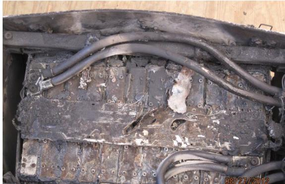
*Burned out lithium-ion battery*
