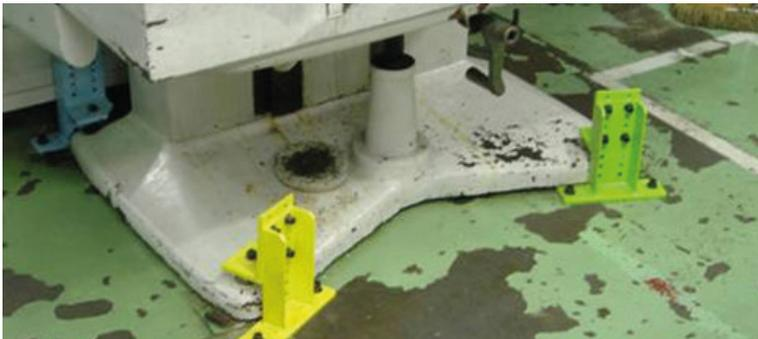
Production equipment anchored to the floor
