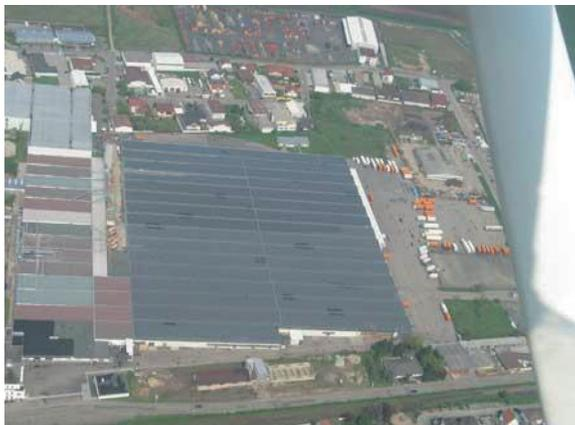
Bürstadt after completion of the installation in 2005 (45 000 m<sup>2</sup>, 5 MW)
