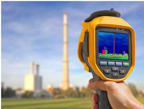
As an object gives off heat, the infrared radiation varies in intensity. By using a specially designed camera the intensity can be displayed visually utilizing various color templates to express the information. The application of infrared technology has been widely used by the military in heat seeking missiles and night vision equipment. Medical and industrial uses of infrared radiation include thermal imaging, or thermography.
